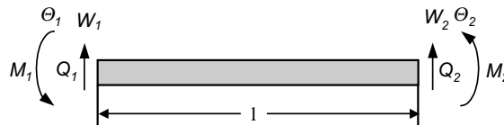
Fig. 1. Sign convention for the moving finite viscoelastic beam element.
